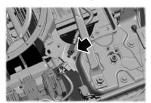
Make the final connection of the negative (-) jumper cable to the negative (-) ground point of the discharged battery vehicle. 5. Unlock the driver door.
