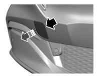
Remove the cover at the front of your vehicle below the headlight. Press firmly on the top right of the covers edge, then pull the raised section on the bottom left toward you.
