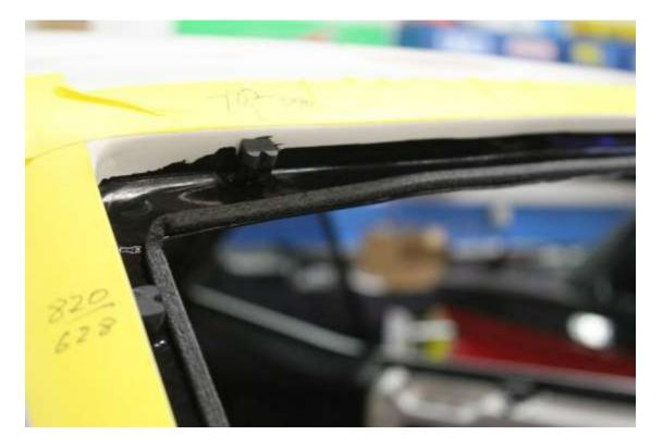
Now for the glass side of the install. Prim the edge all the way around for the urethane. This is a very important step so that the urethane will cure properly.
