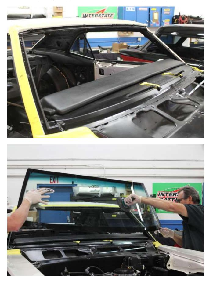
We get asked a lot on how to hold the glass in place so here you go, you can tape the edge down and pull hard to get the glass to flex to where you want it.
