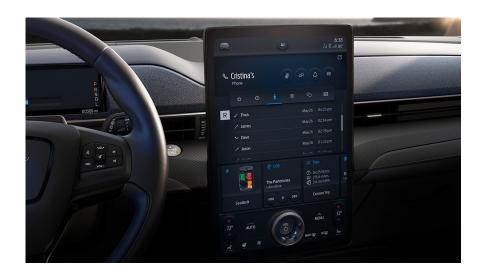
Customers can preprogram their preferred charge times for the vehicle through their FordPass app or the center-stack screen. Remind customers that overnight charging, also known as value charging, is usually the economical way to charge because of lower electricity rates. (5) Mustang Mach-E owners with FordPass can also check their scheduled charge times or active charge status on their phone.
