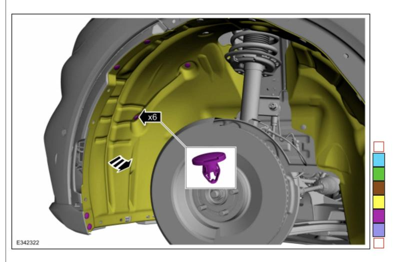
6. Disconnect the camera washer hose and plug the washer hose end. Remove the clips and position the washer hose assembly aside.
