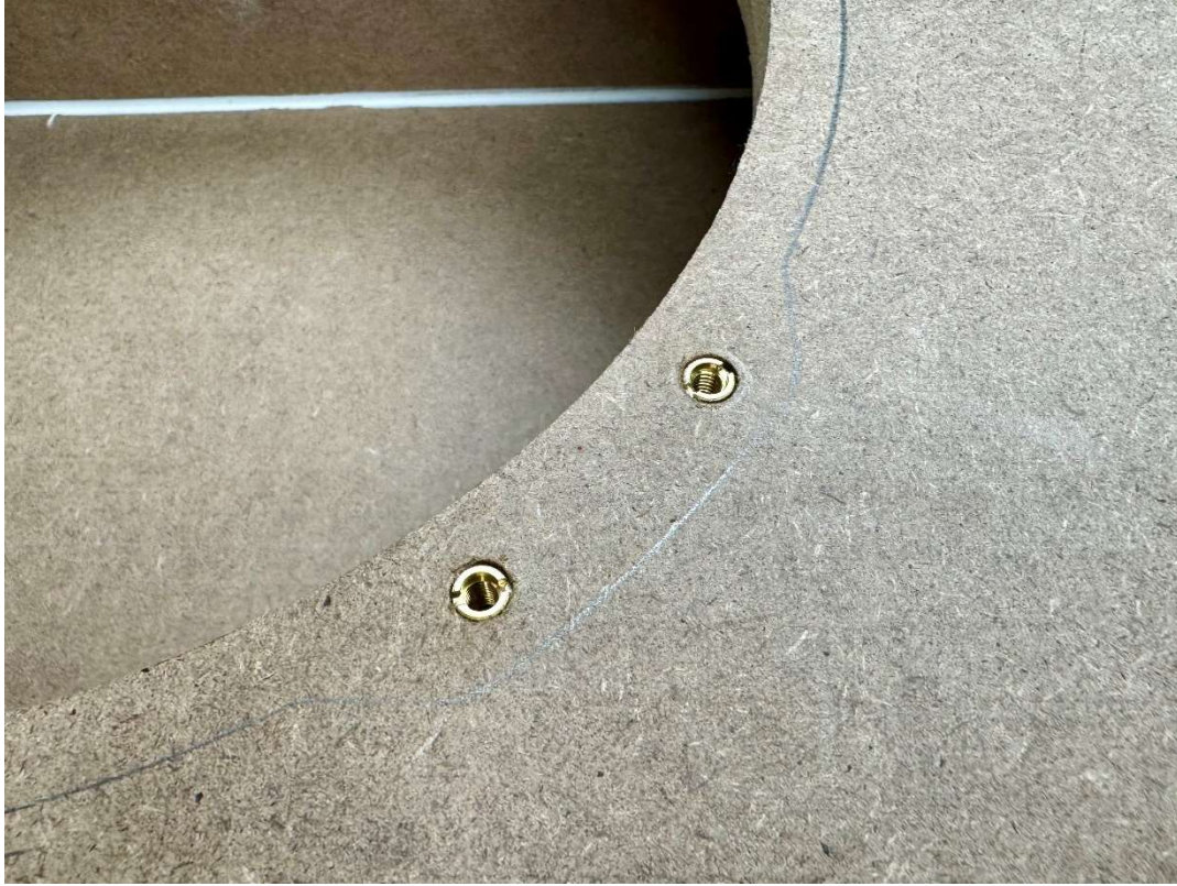
Threaded inserts installed, although I had to back out a half turn once carpet was on for height adjustment.
