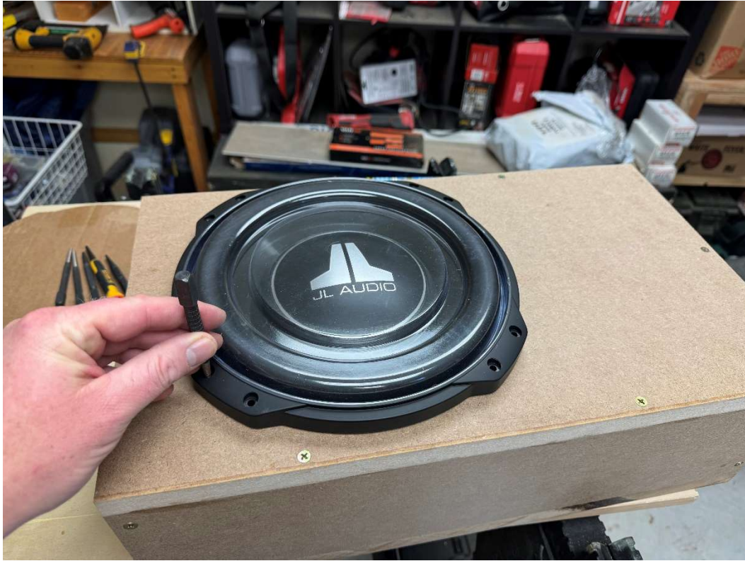
Marking mounting holes with a center punch.
