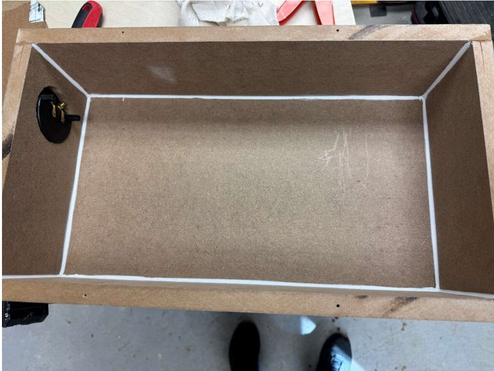
Corner caulking to prevent air seepage.
