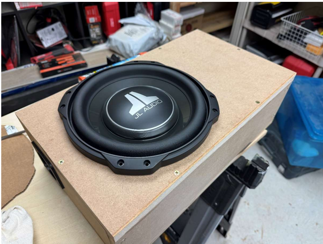
Checking hole fitment. No picture but the hole was cut using a plunging router and a homemade circle jig.
