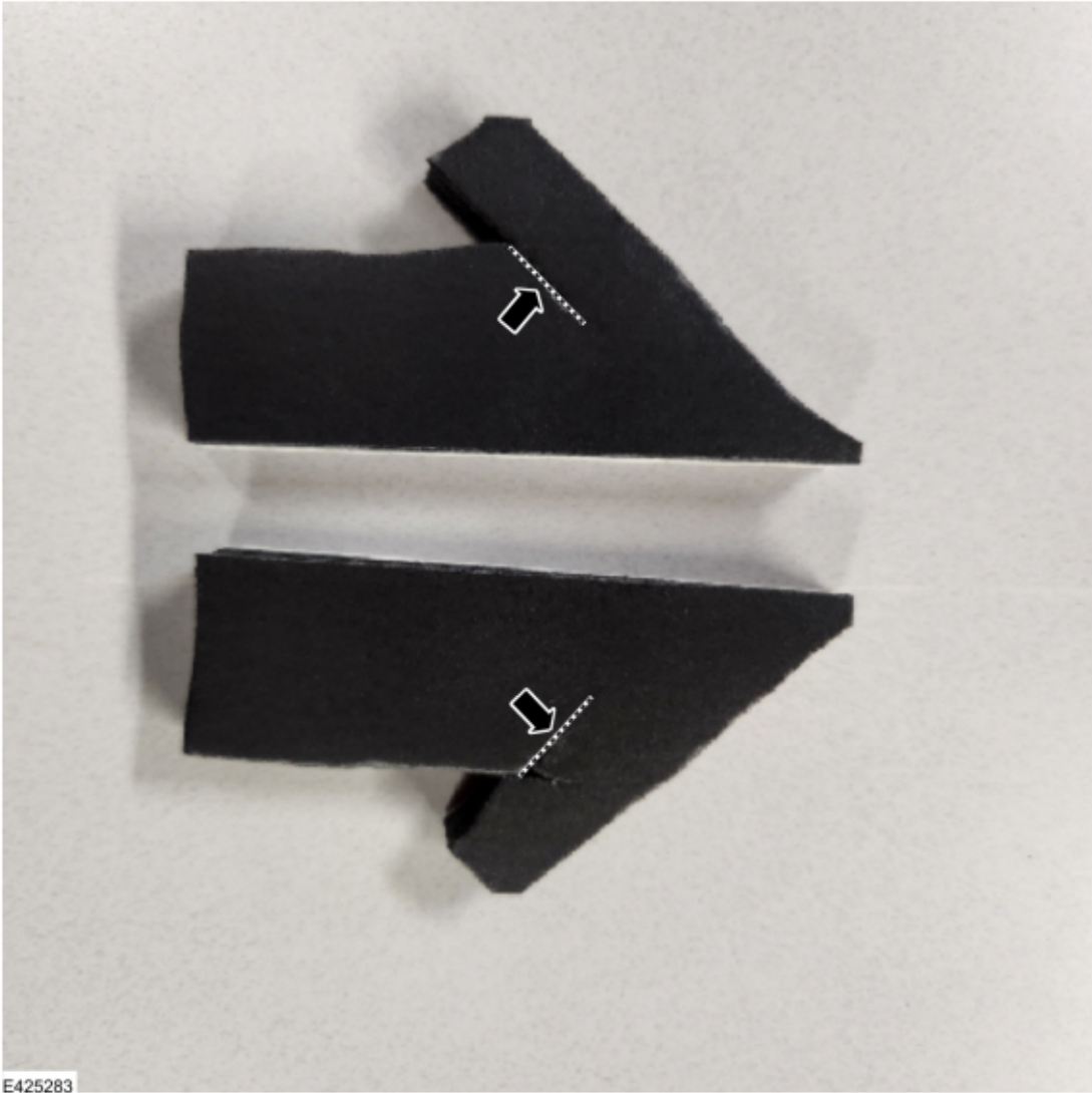
12. Remove the existing glass top run foam and clean the surface to remove any residual foam. (Figures 8-9) Figure 8
