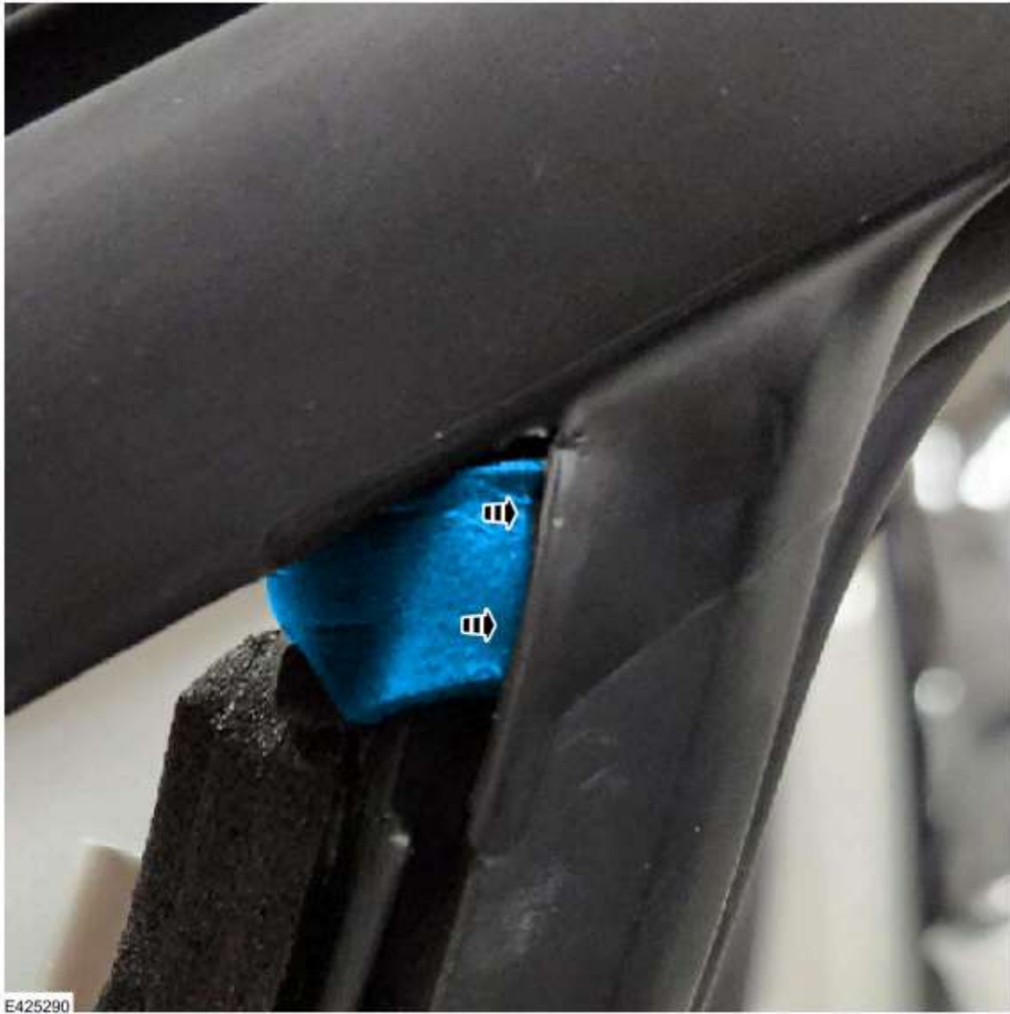
15. Reinstall the front door glass top run in the door frame and the run channel. (Figure 15) Figure 15
